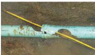
Service lines that have been penetrated during trenchless installation.
