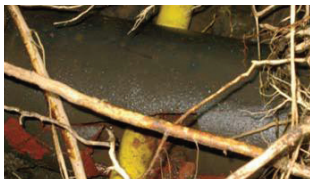
Service lines that have been penetrated during trenchless installation.
